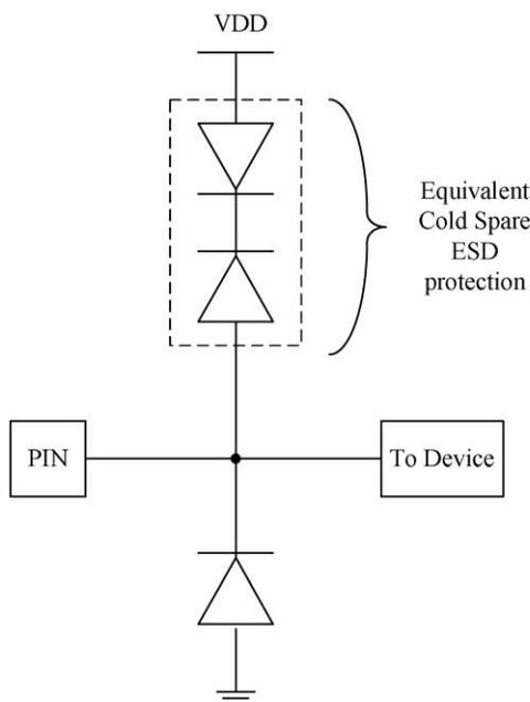
Figure 3. Notional Cold/Warm Spare ESD protection circuit
