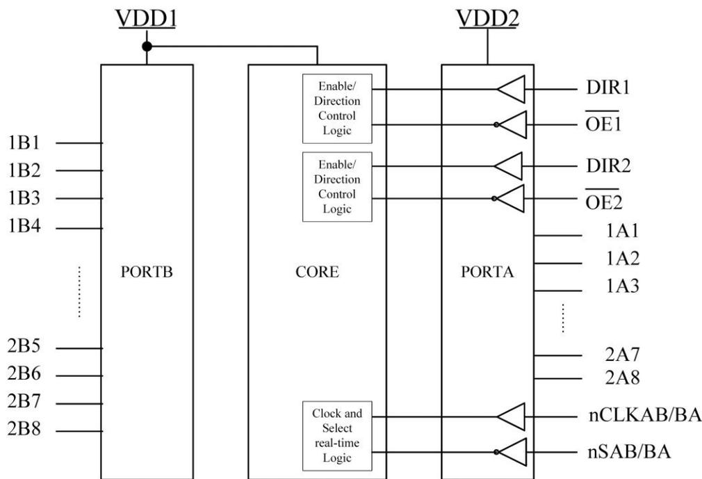
Figure 2. Notional block diagram for UT54ACS164646S
