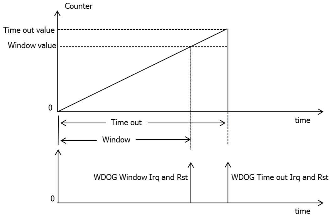
Figure 2: WDOG Time out or Window reset
