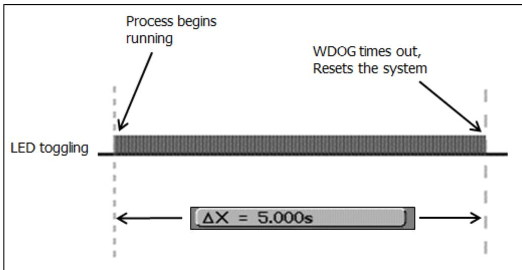
**Figure 3: WDOG 5 secs time out reset**
