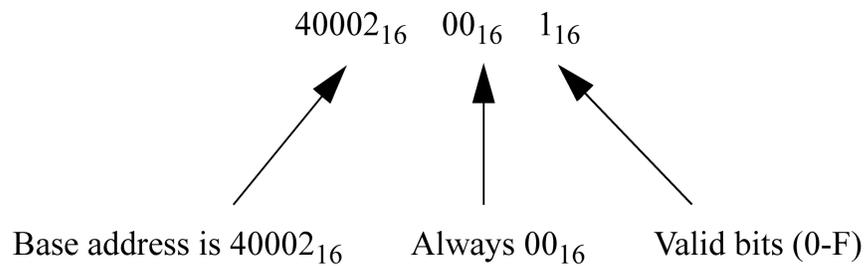
To reconstruct the external address from the cache tag, the DTAG or ITAG field is concatenated with the cache address. In this example, the DTAG field is  $40002_{16}$  and the cache address is  $0000_{16}$ . Therefore, the referenced external address is:
