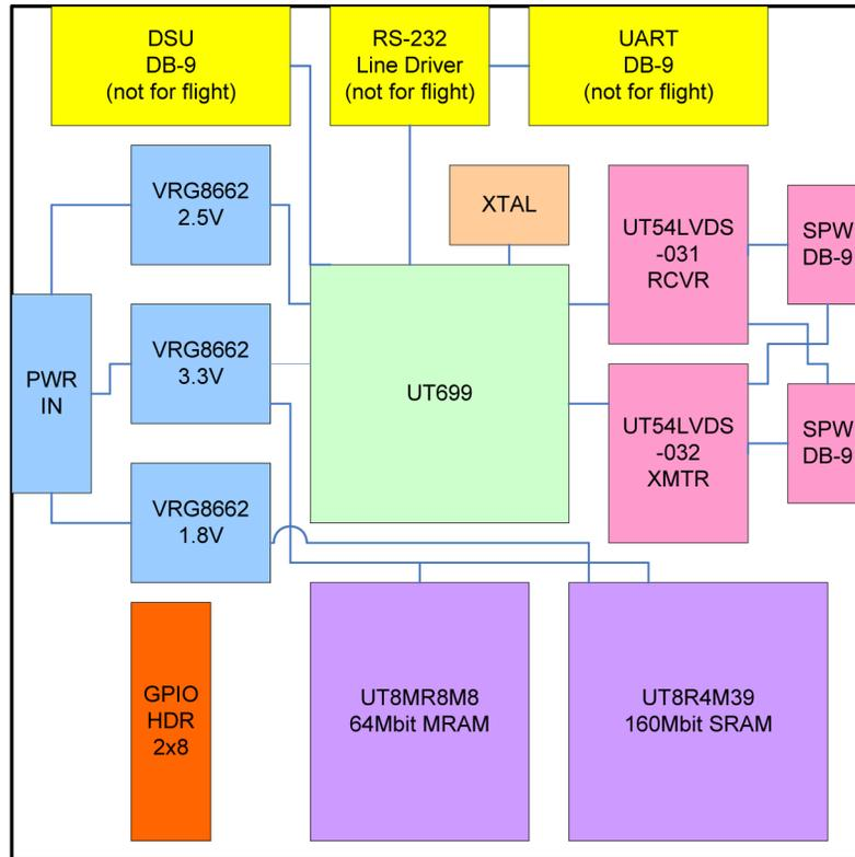
Figure 1. Block Diagram
