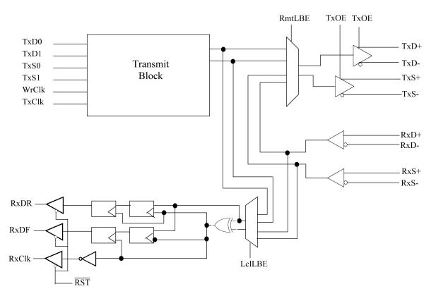
Figure 1. UT200SpWPHY01 SpaceWire PHY Chip Block Diagram
