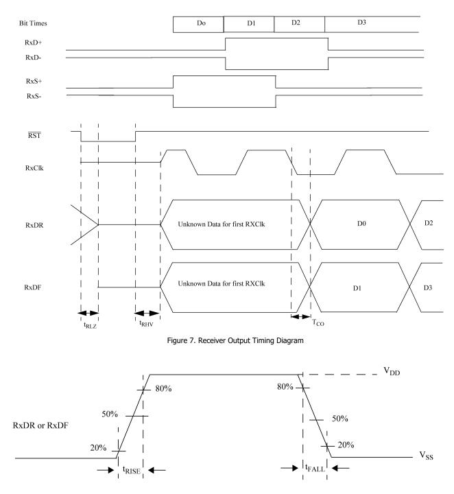
Figure 8. Receiver Output Rise and Fall Times Waveform
