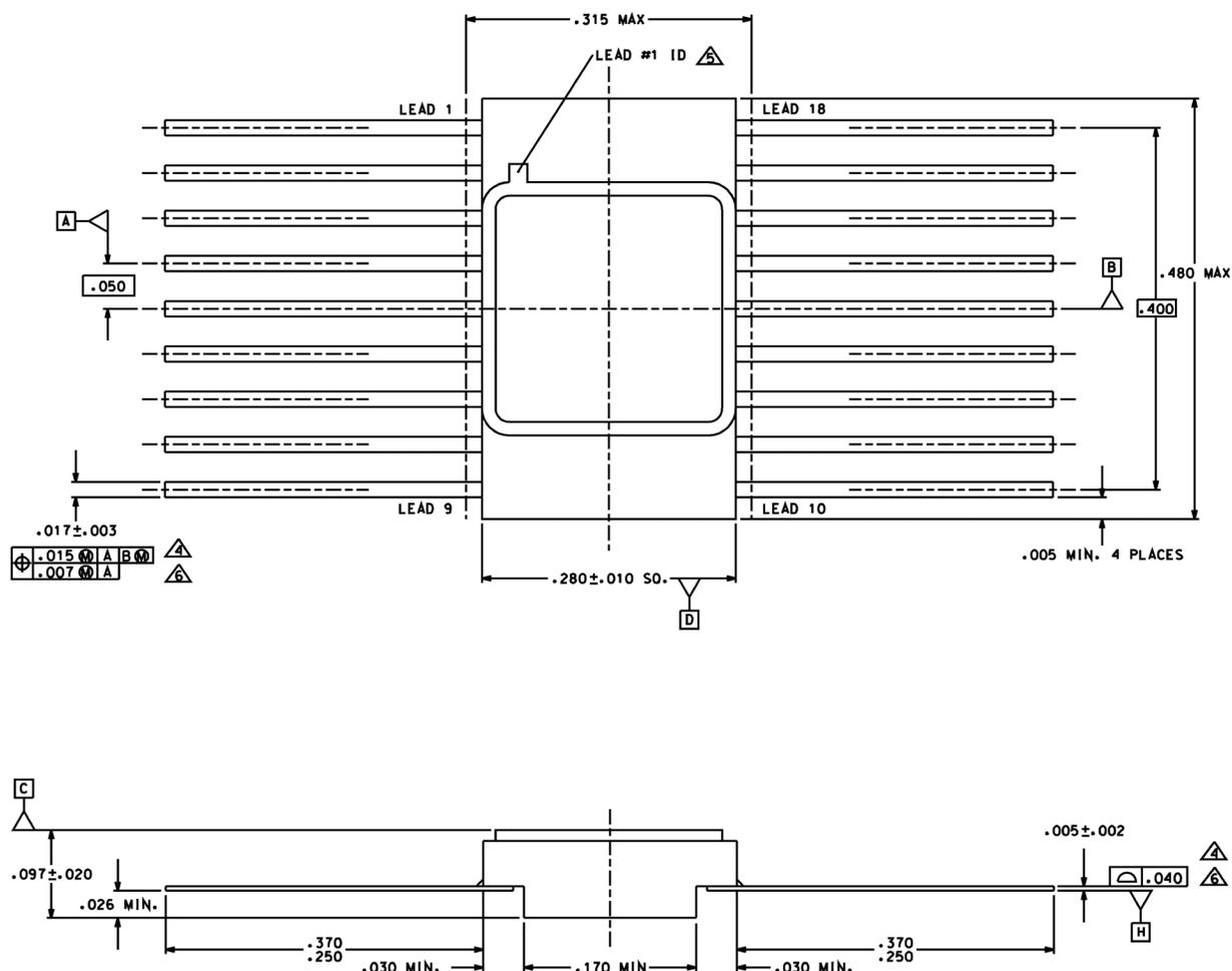
Figure 13. 18-pin Ceramic Flatpack
