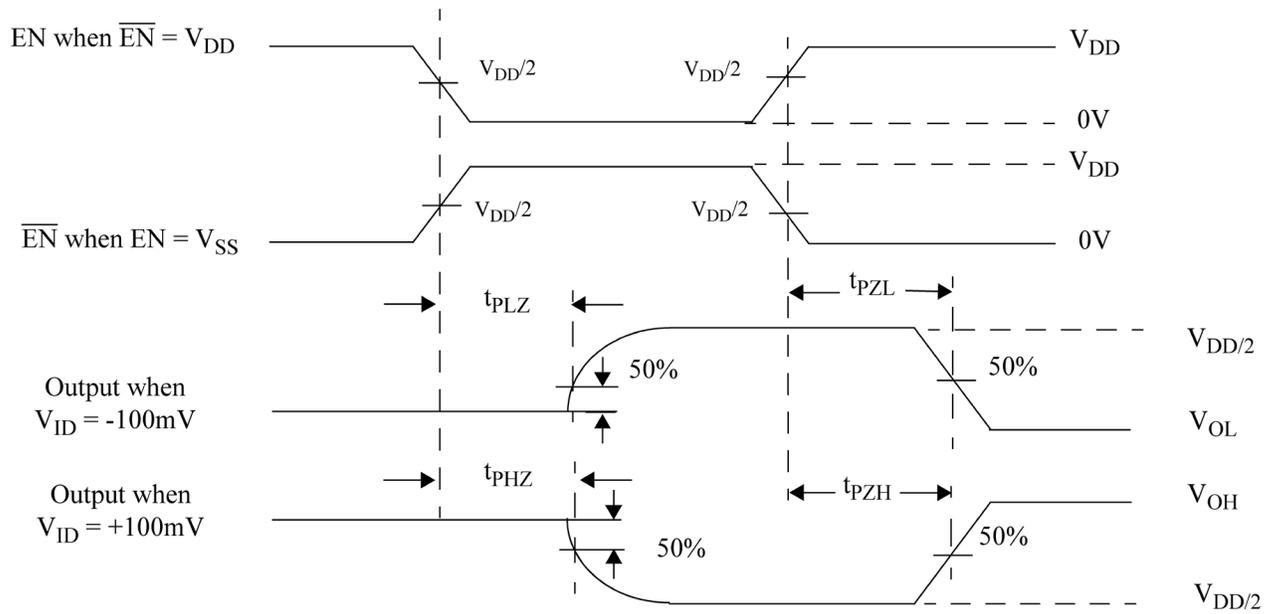
Figure 12. Receiver Three-State Delay Waveform or Equivalent Circuit
