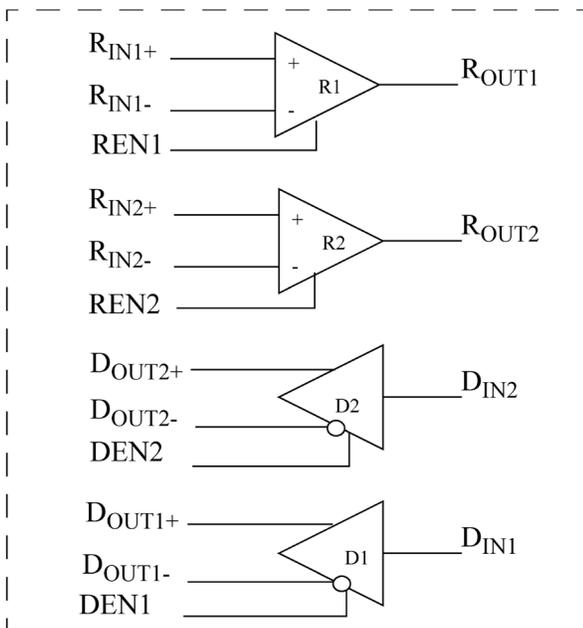
Figure 1. UT54LVDM055LV Dual Driver and Receiver Block Diagram
