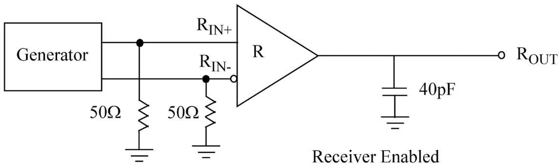
Figure 9. Receiver Propagation Delay and Transition Time Test Circuit or Equivalent Circuit
