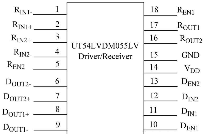
Figure 2. UT54LVDM055LV Pinout
