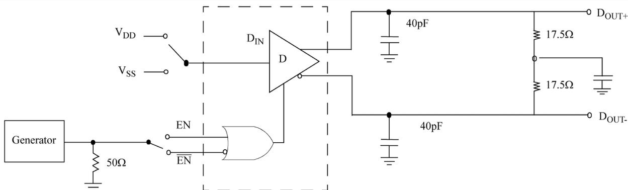
Figure 7. Driver Three-State Delay Test Circuit or Equivalent Circuit or Equivalent Circuit
