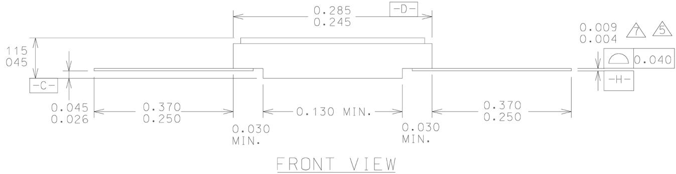
Figure 10. 16-pin Ceramic Flatpack
