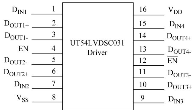
Figure 2. UT54LVDSC031 Pinout
