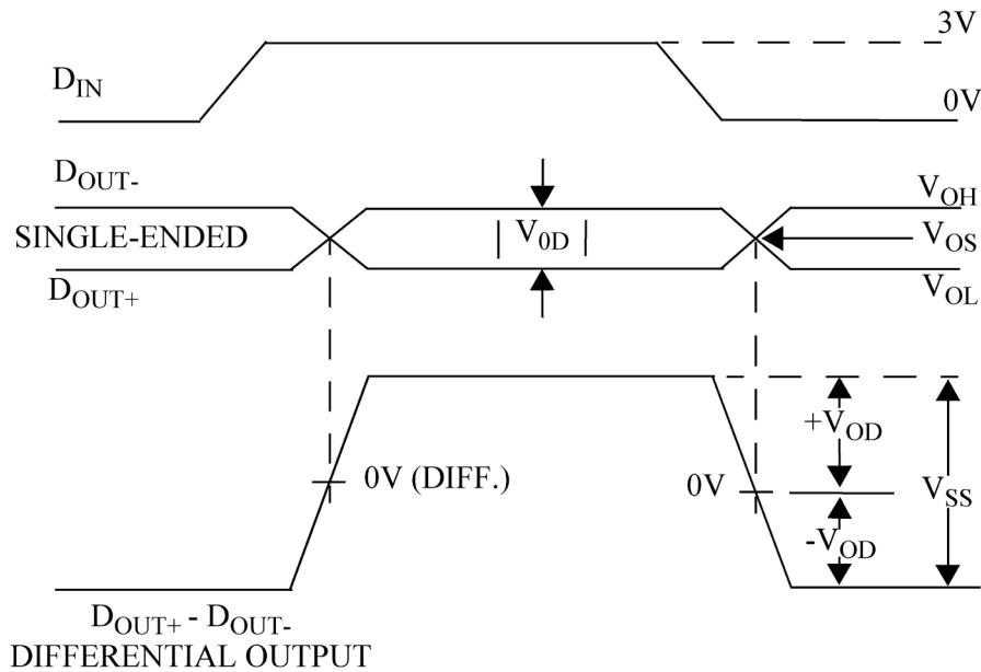
Figure 4. Driver Output Levels
