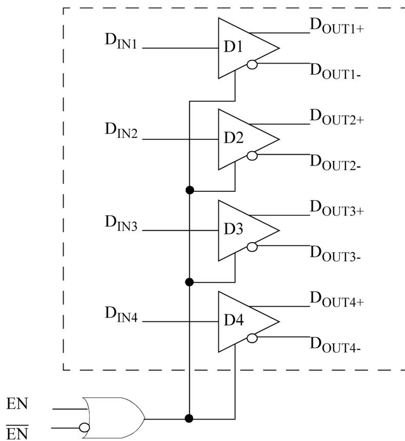
Figure 1. UT54LVDSC031 Quad Driver Block Diagram
