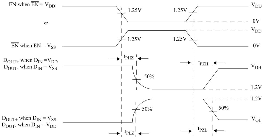
Figure 9. Driver Three-State Delay Waveform
