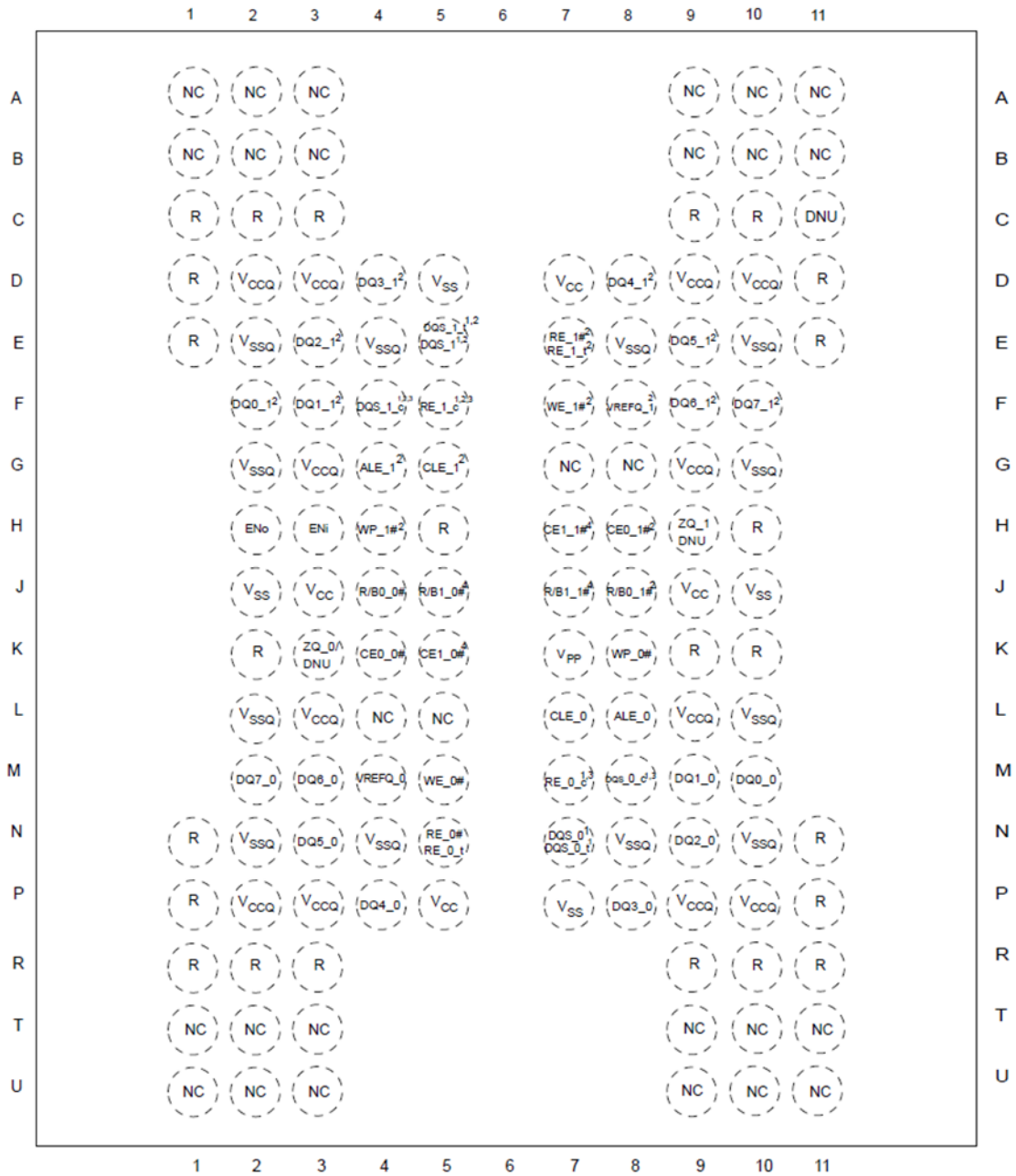
Figure 1: 132-Ball BGA (Ball-Down, Top View)
