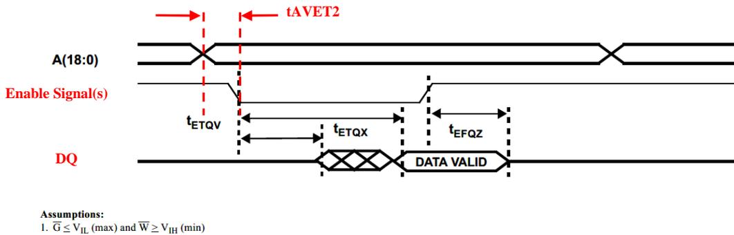
Figure 4b. SRAM Read Cycle 2: Chip Enable-Controlled Access
