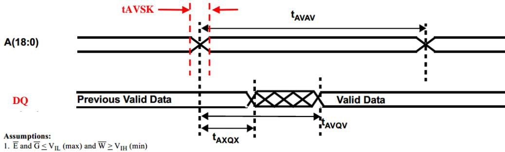
Figure 4a. SRAM Read Cycle 1: Address Access
